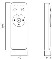
Note: The length L of the remote control depend on product specifications (unit: mm)
