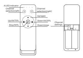
Note: The [channel setting] button is under the cover on the back of remote control
